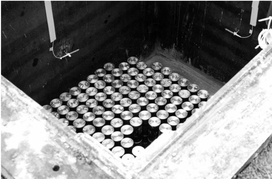
Fig. 10. Experimental setup for spent fuel pool blast test.
